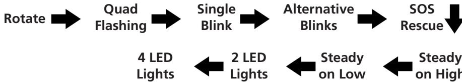
To turn off the warning light without cycling through the 9 light modes, press and hold the power button for 2 seconds. Two LEDs will flash five times and then turn off. When ready to operate again, press the power button once and it will return to the last flash mode that was selected before turning off.
